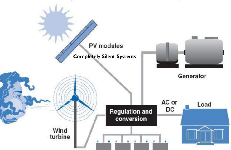
A hybrid system that combines a wind system with a solar and/or diesel generator can provide reliable offgrid power around the clock.
